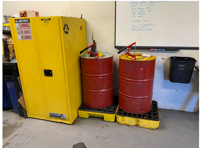
Photo 4: Two 55-gallon drums stored on portable spill containment pallets in the Shop Area
