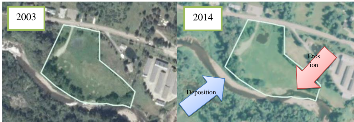
Figure 1. River channel before (left) and after (right) 2013 flood which deposited sediment along the western portion of the Property and eroded riverbank from the eastern portion.
